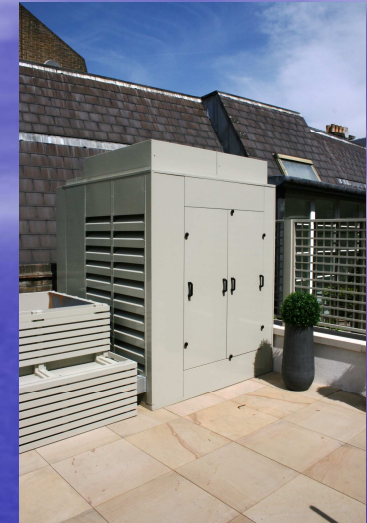
Acoustic Louvred Enclosure designed for vertical discharge air cooled condensers and heat pumps c/w mid-range performance inlet and discharge acoustic louvres & AP50 Acoustic Panels & removeable access panels
